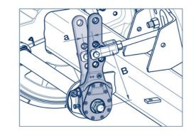
E.g if brake lever length = 10 mm, then set play =15 - 18mm. **Note: Slack adjuster should be approximately 90° to each other when using the brakes** If unsure of the procedure please contact Mehvar Sazan Chichest Chichest Transpec.
