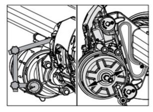
Press the brake caliper upwards and determine the play of the bearing on the dial gauge.
