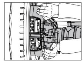
The bearing play of the brake caliper can be determined using a dial gauge. Attach the dial gauge holder to the axle beam and position the gauge on the brake caliper housing on the brake cylinder holder.
