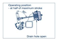
Depress the clutch sleeve around the adjustment screw. Turn the adjusting screw to line up the clevis pin hole to the relevant slack adjuster hole. Ensure that the pushrod has been cut to the correct length.
