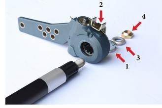
retaining nut to 80 - 90mm ensuring that the brake lining wear indicator is pointing vertically up! Fit the anchor brakes and leave the nuts loos at this stage.
