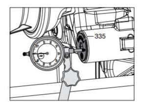
clearance readjusted. Use a dial gauge to determine the clearance. For this purpose, attach a dial gauge holder to the axle beam and position the probe on the outside of the fixed bearing scaling cap. If the clearance is not within the tolerance, the adjustment and the brake caliper guide should be checked.
