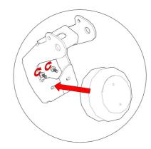
To install the movable arm of the lifting set, place it on the convoluted air spring from the opposite side and use two bolts (hexagon head bolts M10x1.530-) with 2 washers in place and close it by hand and connect it with the moving part by two screws (hexagon head screw M16x2 - 40mm) with two nuts (hexagon nut and washer M16x2).
